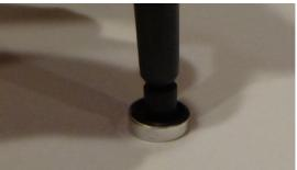
3) You can also use tweezer probes to form lid around sample CAUTION: Pressing too hard with tweezers can deform bottom of pan
