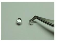
3) Using the flat end for films, fibers and powders and the concave end for other samples, firmly press the cover down into the pan with the Hand Press Tool. \*Both the pan with flange and the pan without flange are compatible with the TA Tzero crimper with the "Press-to-Fit" cover. Pressing force is stiff but not difficult.
