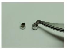
3) Using the flat end for films, fibers and powders and the concave end for other samples, gently press the cover down into the pan with the Hand Press Tool. The cover is soft and will typically form around your sample so there is no need to press hard.
